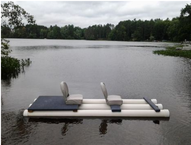
PVC Raft - alternative to a wooden frame, use PVC-pipes of various sizes and diameters.
